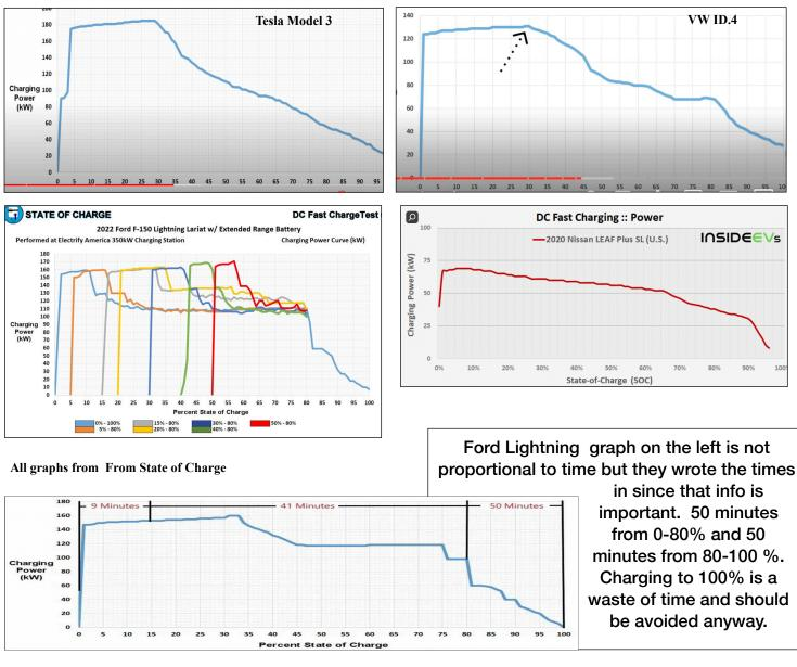
In the graph on left has two different charging times. 20 minutes going from 30% to 70% and 57 minutes from 20% to 100%. Charging 20 minutes twice (or 40 minutes) saves 17 minutes at the charger with the benefit of getting another break for restroom and stretching legs.
