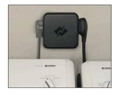
Share an outlet: e.g. Plug in two things. If device on primary outlet is not in use (in this case dryer), the second outlet goes live. I made access so the electric dryer outlet adjacent to my garage can be used for EV charging. It is very important that such devices are UL approved. Cheap ones won't handle the electric load.
