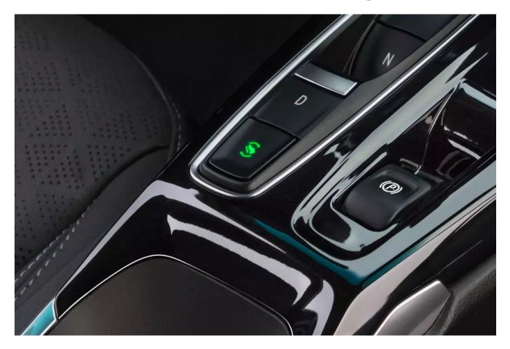
One-pedal driving is a feature on some electric vehicles where, under most circumstances, you use only the accelerator pedal to both speed up and slow down. When activated, the brake pedal only comes into play if you need to make a hard stop.
