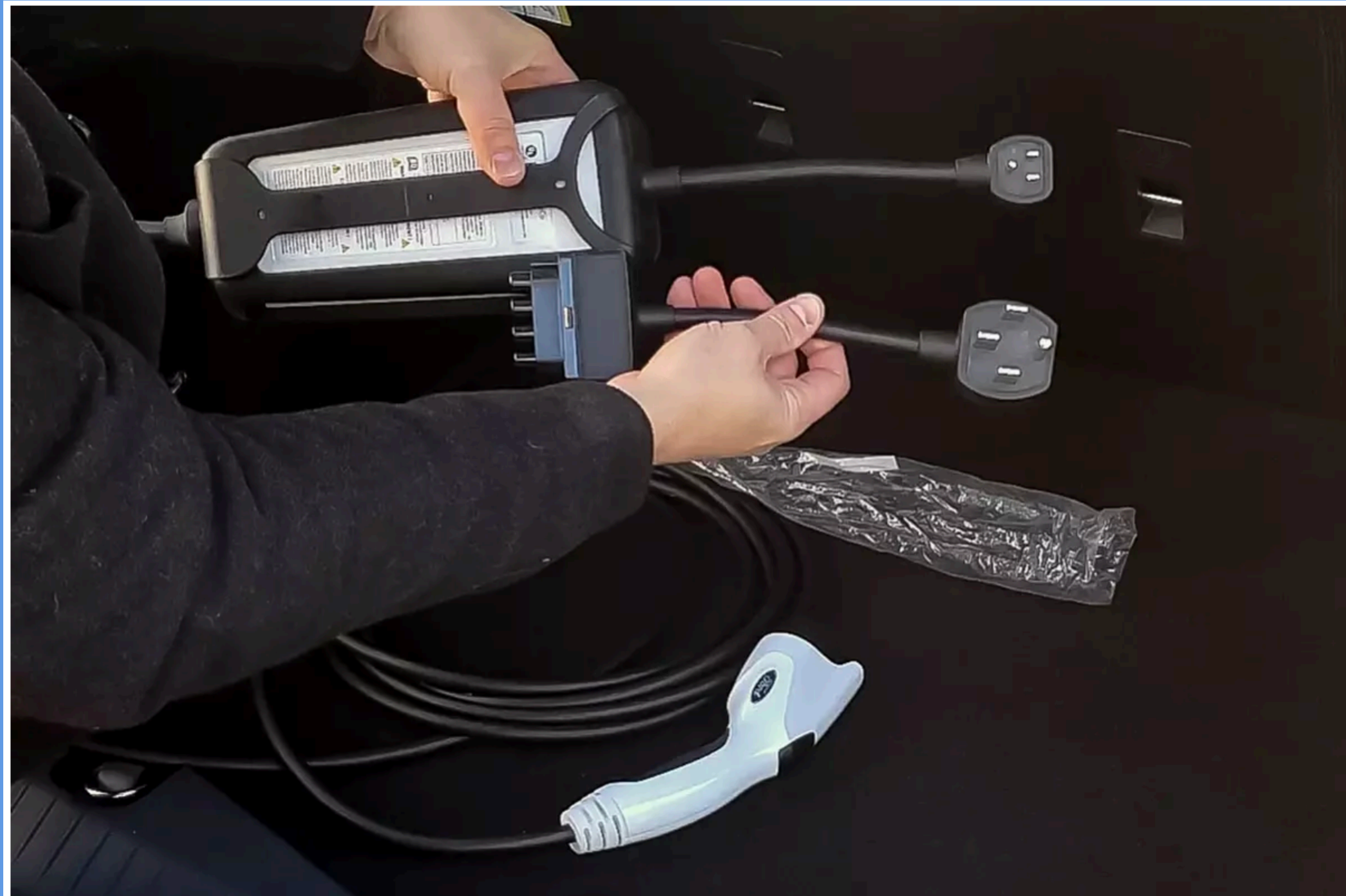
Ford Mustang Mach-E's supplied charger with interchangeable 120- and 240-volt plugs | Cars.com photo by Joe Wiesenfelder
