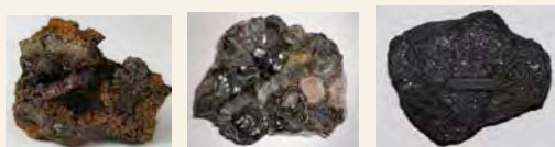
Three different types of iron ore (l. to r.): limonite, goethite, and magnetite
