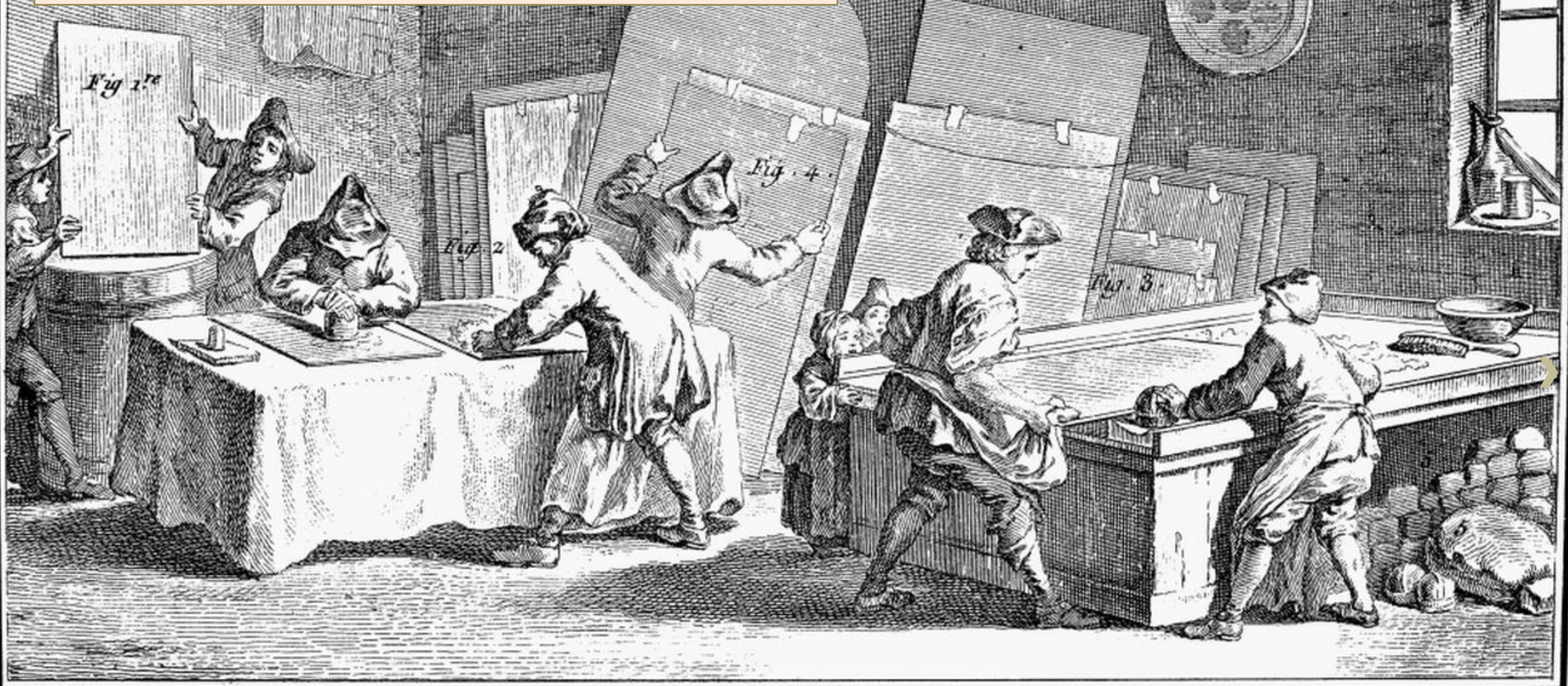
Coating large plate glass mirrors with Tin-amalgam 'tain' France, mid 18 th Century
