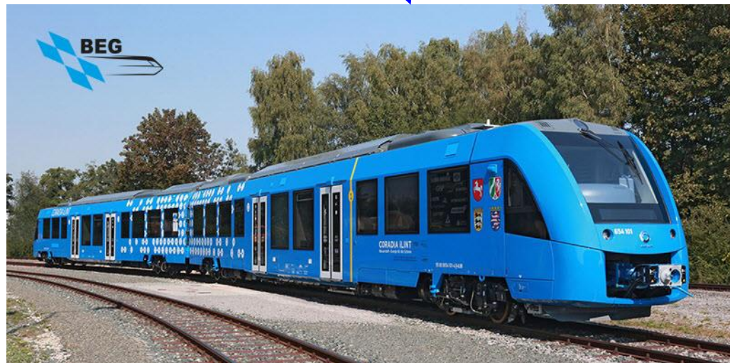
Alstom Hydrogen Fuel-Cell Train (Austria) 600km range, 140 km/h speed
