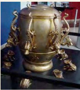
Model of a Chinese seismometer from the Han Dynasty period
